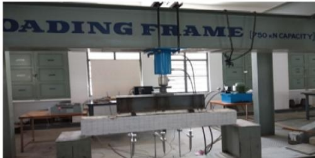
Fig.5 Schematic arrangement for testing of a RC beam
