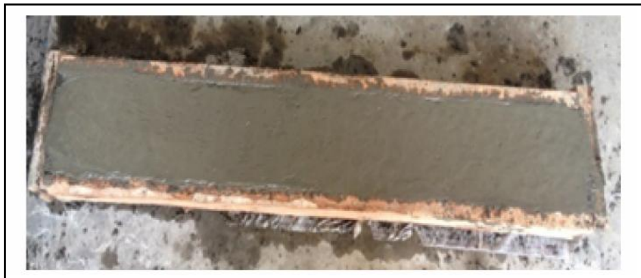
Fig.7 Casting of beam
